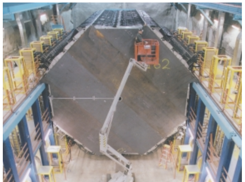
The two supermodules that will detect neutrinos arriving at the lab weigh 6,000 tons, equivalent to a total of about 5,820 Ford Taurus cars. Iron ore for the 486 steel planes inside the detectors comes from Hibbing Taconite.
